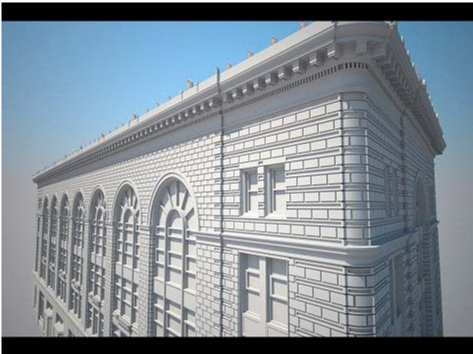
A final rendering of the Mariner building in Autodesk Maya. Matt Wright comments about the photogrammetry process: "One thing that we learned very quickly was that photogrammetry is very different to regular photography, or even photography for texture/reference work. You constantly have to think about angles between camera shots, what you have in frame, making sure there is enough detail and depth in the image."
