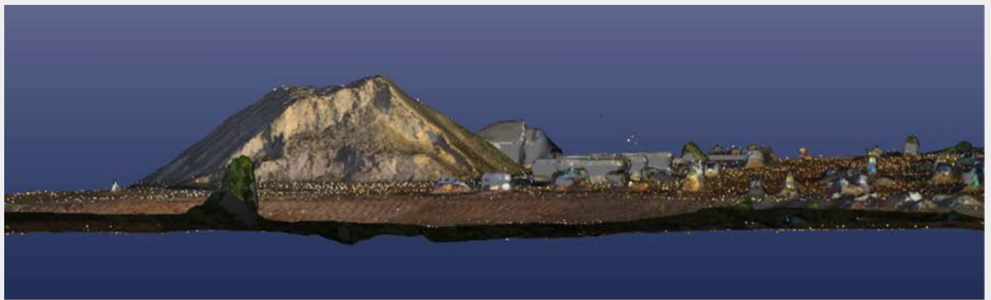
Figure1: 3D model produced from PhotoModeler and drone photography as basis for stock pile volume measurements
