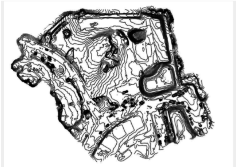
Figure 2: One-foot contour map produced from PhotoModeler and drone photography on a Sullivan Eastern, Inc project site.
