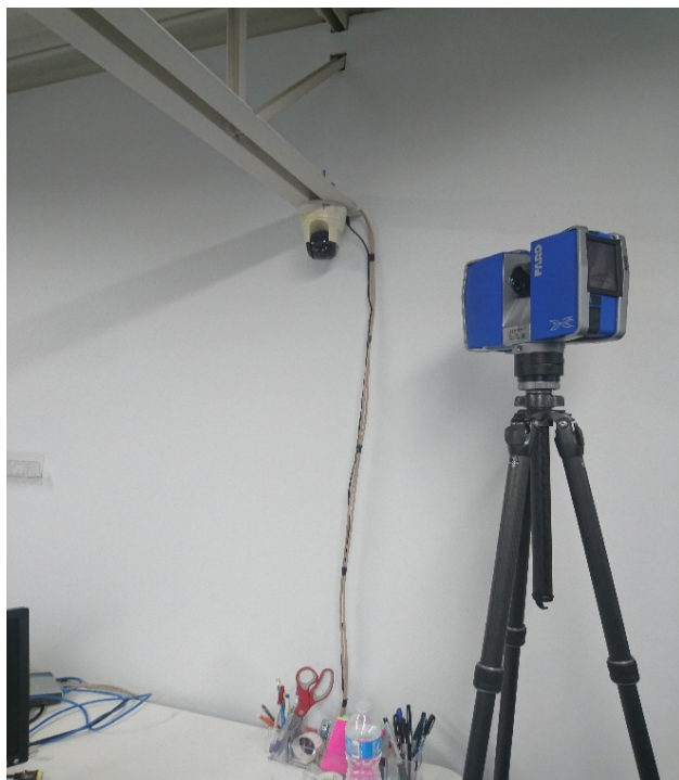
Figure 2. Faro laser scanner positioned close to the cameras position to provide similar field of view for matching common reference points between the security camera image and the laser scan data.
