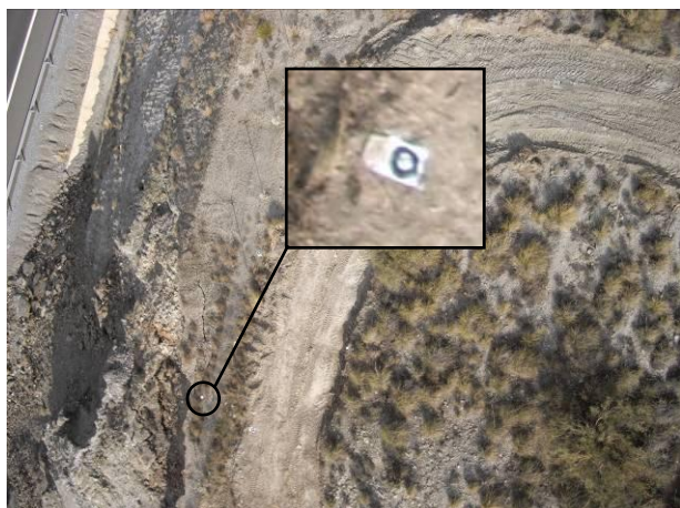
Figure 13. Detail of one of the 29 target points zoomed from a photo of the photogrammetric project
