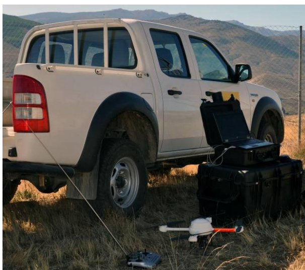
Figure 1. Microdrone UAV, base station and hand held remote control transmitter
