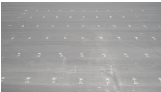
Figure 4. Field calibration surface with the targets points
