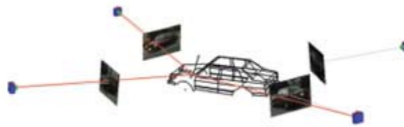
Figure 1: Import overlapping bitmap images into PhotoModeler 6 that show the object from as many sides as possible, and you can reverse engineer anything.
