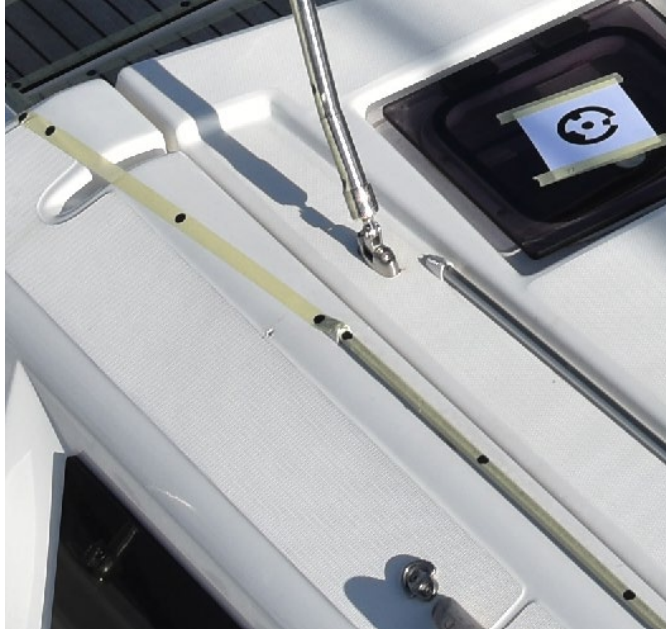
Example of dot tape on deck and dot targets on the track for bottom of sprayhood/dodger canvas. Project data courtesy of Dustom d.o.o. ( Dustom Covers ).
