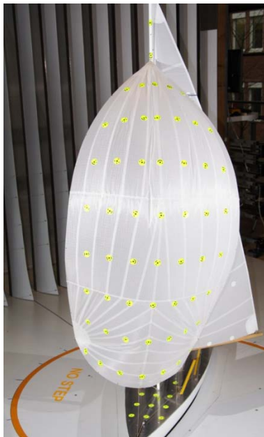
Fig. 5-3: Symmetric spinnaker equipped with 55 coded targets
