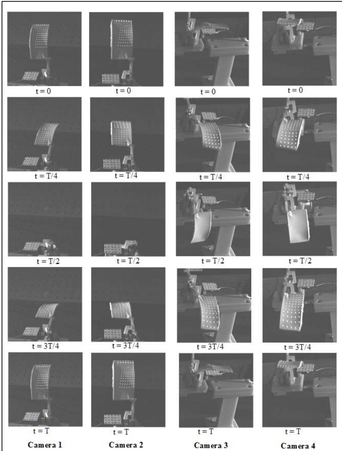
Figure 62: Images of Curved Tube Frame Wing flapping at 6.2 Hz
