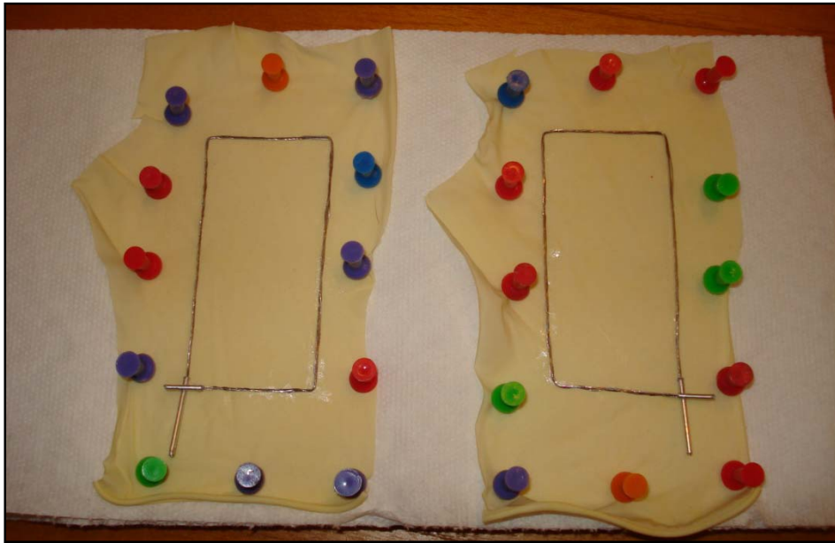
Figure 23: Attachment of Latex Membrane to Wing Frames
